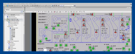
Automation,Installation and commisioning of beer packaging line from packer,conveyor,bottle washer,filler and labeller using s71500 PLC and wincc confort SCADA
