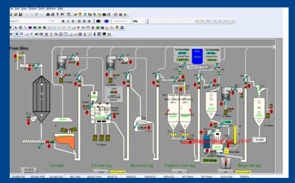
• PLC and SCADA design and installation using S7300 PLC and CX supervisor SCADA, field wiring, electrical system installation and termination, and commission of 120T/H grain cleaner, destoner, degermer and milling machines
