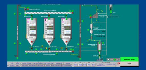
• PLC and SCADA design and installationusing S7300 PLC and WINCC SCADA, field wiring, electrical system installation and termination, and commisioning oF 60 T/H bulk loading facility in maltings section
